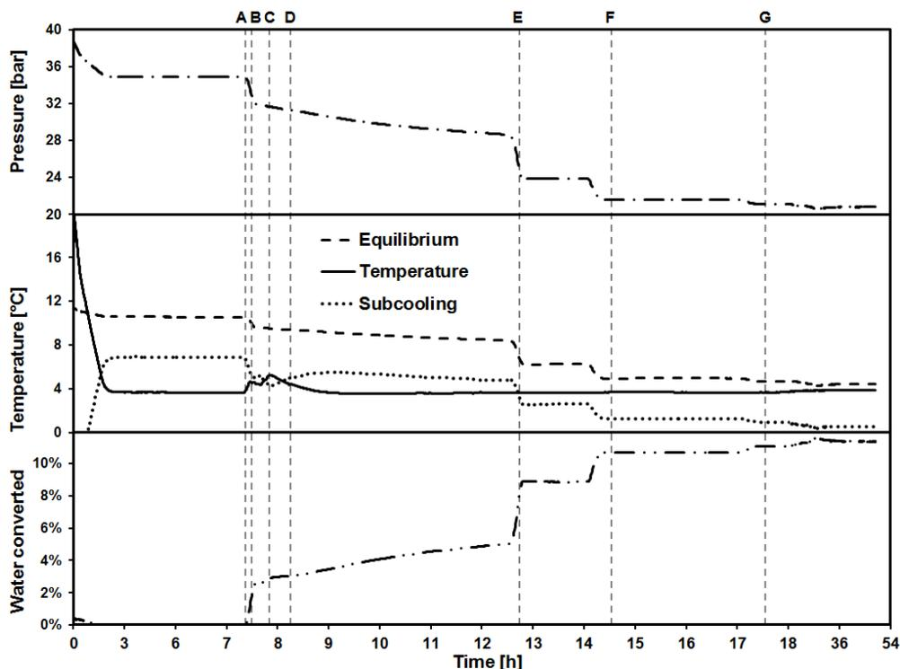
Figure 2. Measured and calculated results from a rocking cell experiment with observations during the experiment. The vertical dash lines A to G in the plot refers to specific key mechanistic events observed related to hydrate formation during the experiment. Time axis is compressed before 6 h and after 18 h for clarity.
