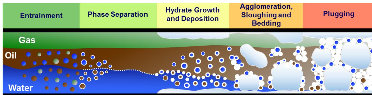
Figure 8. Revised conceptual model for hydrate formation and accumulation in shear stabilized dispersion (non-emulsifying oil).
