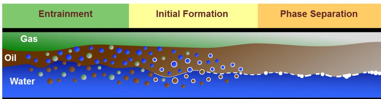
Figure 5. Steps leading to phase separation: Entrainment: phases are dispersed before hydrate formation due to shear forces from the flow; Initial Formation: hydrates form at all hydrocarbon-water surfaces; and Phase Separation: hydrate formation causes the liquid hydrocarbon and water phases to separate in flowing conditions.
