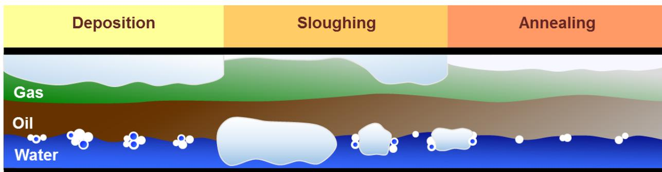
Figure 6. Illustration of hydrate formation and accumulation observed in the experiments. Initial formation of hydrate deposits of high volume and porosity at high subcooling. Sloughing, and Annealing or formation of deposits with lower volume and porosity at conditions close to hydrate equilibrium.
