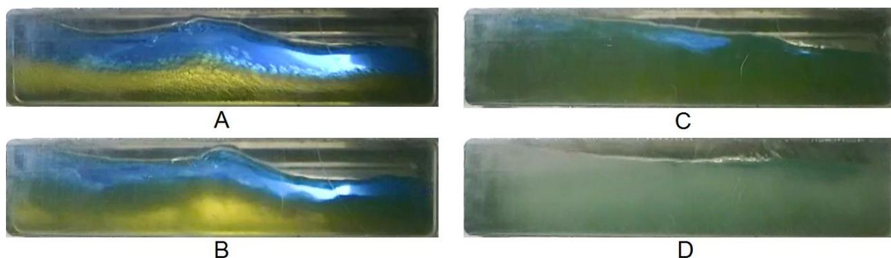
Figure 4. Before hydrate formation: (A) Condensate (blue) and water in oil dispersion (yellow). Various stages of the hydrate formation: (B) Hydrates can be seen as particles at the water/condensate interface 30 seconds after hydrate onset, (C) dispersion of hydrate particles in water, and (D) a solid hydrate deposit.
