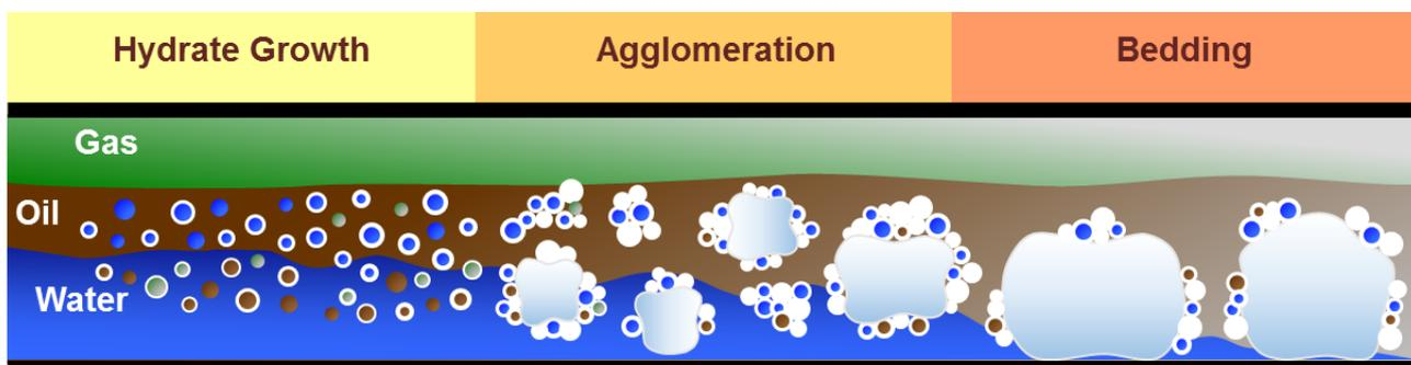
Figure 7. Steps in formation, agglomeration, and accumulation of hydrates as observed in the rocking cell experiments for predominant bulk hydrate.
