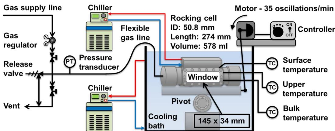
Figure 1. Schematic of the experimental setup for the rocking cell system for hydrate experiments.
