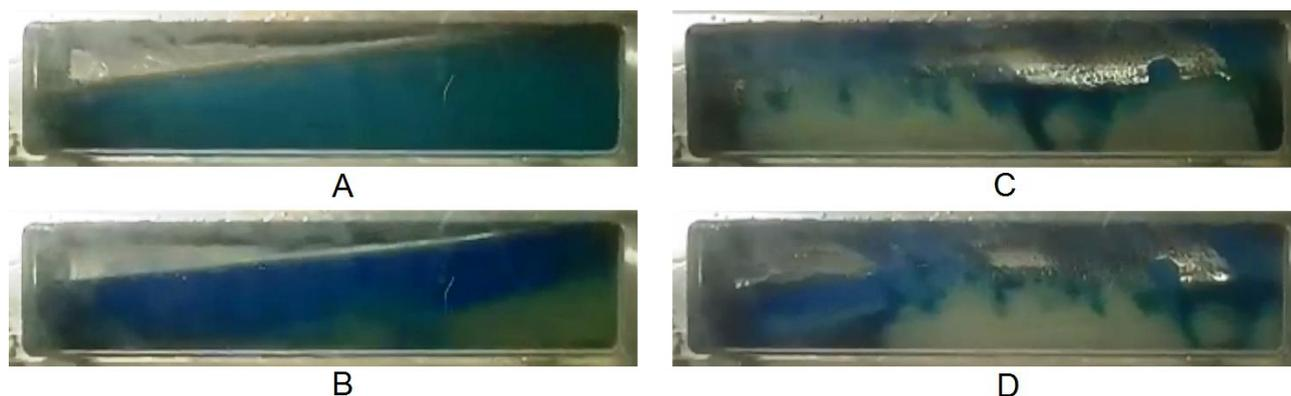
Figure 3. Phase separation: (A) Dispersion before hydrate formation started. (B) Phase separated oil (blue) and water (yellow) 4 minutes after hydrate formation onset. Sloughing and bedding: (C) Hydrates attached to the surface in the upper left part of the window, (D) sloughed off the wall and entered the oil phase with bedded hydrates.
