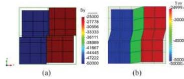
Figure 13. XX-Stress variation for Case-2. (a) Discrete IE-FEM (b) Multilaminate model.
