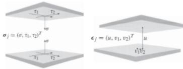
Figure 4. Stresses and relative displacements in zero-thickness interface element formulation (IE-FEM). Adapted from Garolera et al., (2013).
