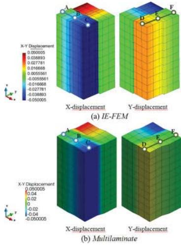
Figure 7. Lateral displacements for case-1 (deformed mesh with 10x factor). (a) Discrete IE-FEM, (b) Multilaminate model.
