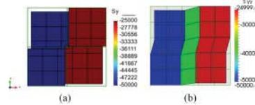
Figure 9. YY-Stress variation for Case-1. (a) Discrete IE-FEM (b) Multilaminate model.
