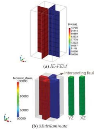
Figure 14. Normal stress on fault planes for Case-2. (a) Discrete IE-FEM, (b) Multilaminate model.
