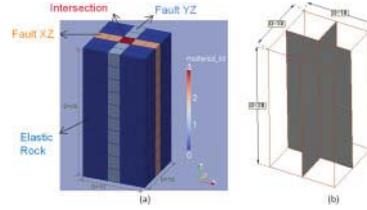
Figure 5. FE Geometry of example 1: (a) Multilaminate material to represent intersecting faults; (b) Fault planes in IE-FEM.
