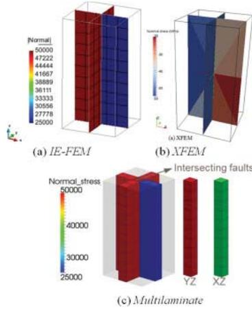
Figure 10. Normal stress on fault planes for Case-1. (a) Discrete IE-FEM, (b) Discrete XFEM and (c) Multilaminate model.
