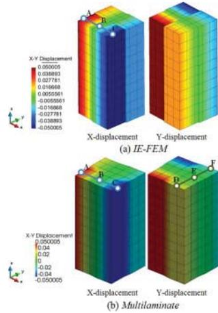
Figure 11. Lateral displacements for Case-2 (deformed mesh with 10x factor). (a) Discrete IE-FEM (b) Multilaminate model.
