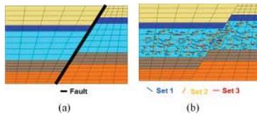
Figure 17. (a) Fault representation using XFEM. (b) Fracture set representation using Multilaminate model.
