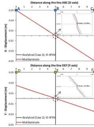
Figure 12. Lateral displacements along the lines ABC and DEF (Figure 11) for Case-2 (inset showing zoomed view of displacement jump on faults). (a) X-Displacement, (b) Y-Displacement.
