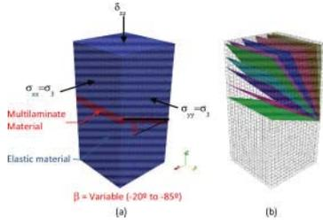
Figure 15. FE Geometry: (a) Multilaminate material; (b) Fault planes with different angles in XFEM.
