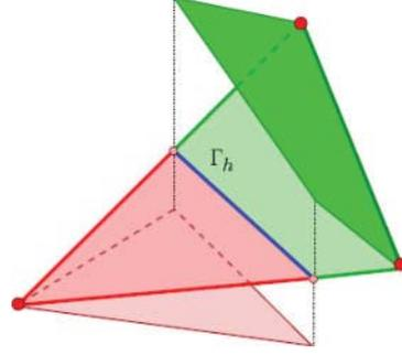
Figure 2. Sum of the nodal enrichment functions in a typical triangular element cut by the interface  $\Gamma_h$ .
