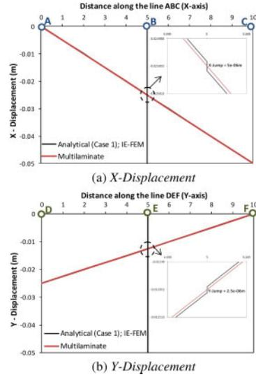
Figure 8. Lateral displacements along the lines ABC and DEF (Figure 7) for case-1 (inset showing zoomed view of displacement jump on faults). (a) X-Displacement, (b) Y-Displacement.
