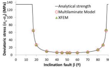
Figure 16. Comparison of Fault strength obtained from analytical solution and XFEM and multilaminate analyses.
