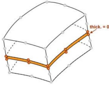
Figure 3. Zero thickness interface element inserted into the continuum FE mesh.
