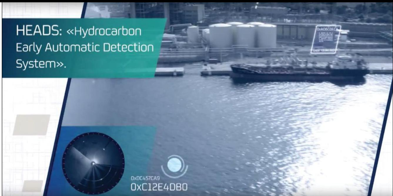
*HEADS consists of oil-detecting infrared cameras, oil spill detection radar, and two control algorithms. The first algorithm detects the oil spill and sets off an alarm through the infrared sensors. The second integrates the signals of both sensors and—based on these signals and the weather conditions—decides whether to set off the alarm to signal an oil spill.*
