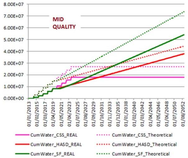
Figure 15. Cumulative injected water – MQ sector
