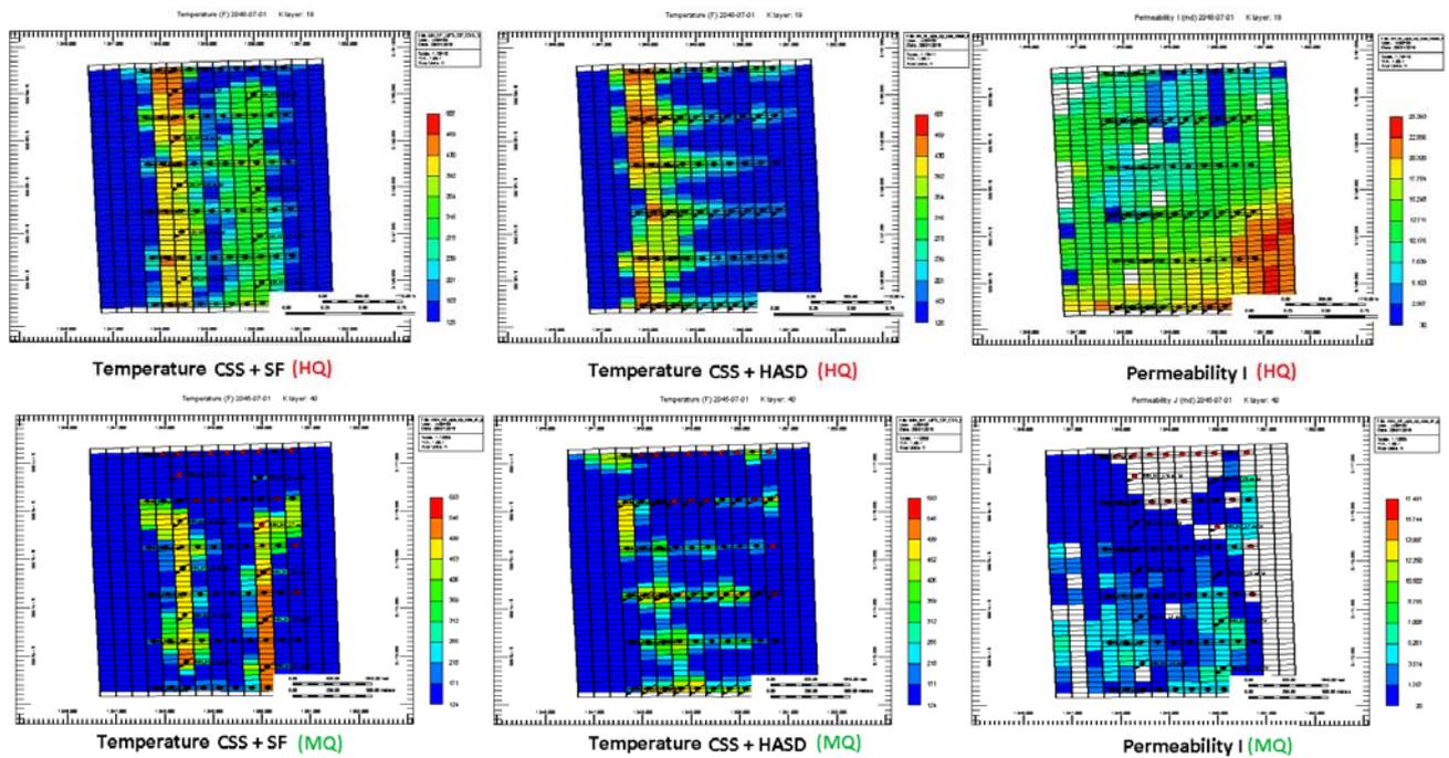
Figure 19. Temperature distribution around producers after 25 years of HASD/SF operation (top: HQ; bottom: MQ)
