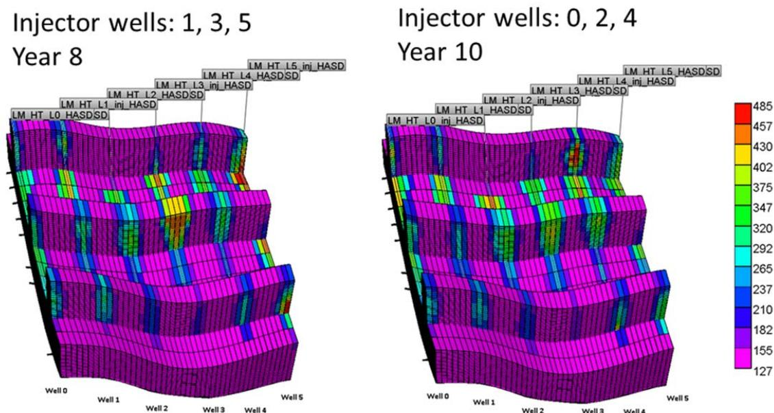
Figure 1. Temperature at two different moments of the HASD cycle
