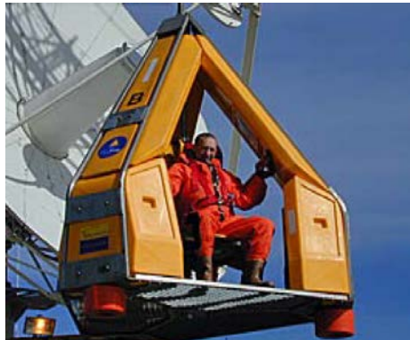
Figure 5. Personnel transfer using a personnel transfer capsule
