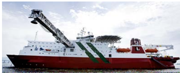
Figure 8. Personnel transfer using a hydraulic bridge
