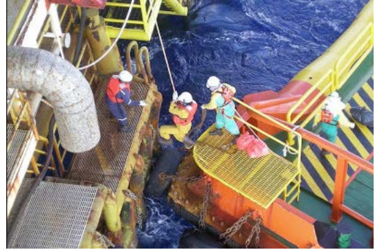
Figure 9. Transferring workers via swing ropes, in the Gulf of Guinea area
