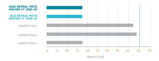
The results obtained for the two Repsol products as well as for competitor 3 are very similar and have a notably higher quality versus competitors 1 and 2. Values are less than half of the strict limit set by API SN.
