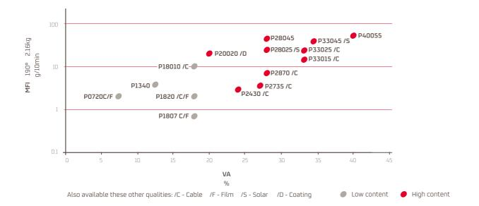
These base resins are suitable for the fabrication of halogen-free flame-retardant (HFFR), semiconductive or other cable compounds
