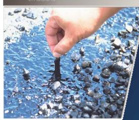
**Modified Emulsions** are colloidal dispersions of globules of bitumen premodified with polymers within an aqueous phase or conventional bitumen emulsions modified with latex.
