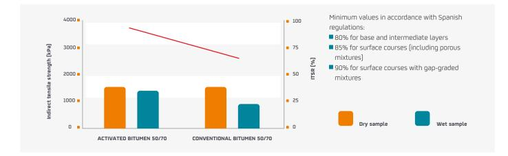
Water sensitivity test results [EN 12697-12] (AC22G mixture, with a porphyry aggregate and 4.1% bitumen 50/70 without additives). These values are illustrative and not binding, nor subject to specification.
