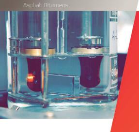
**Asphalt bitumens** are hydrocarbonated binders resulting from the distillation of oil, with viscoelastic behaviour depending on the temperature and high chemical stability. They are also called penetration grade bitumens as it is this property by which they are classified.
