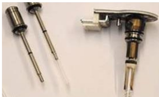
Pyrolysis module with Platinum filament, transport adapters and sample holders (Gerstel)
