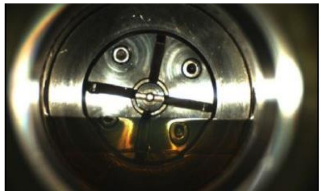
Visualization of liquid-vapor interface in PVT Test. The cell comes with an interpretation software to establish volumetrics
