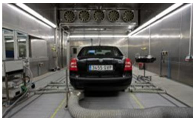
Vehicle chassis dyno and climatic chamber image
